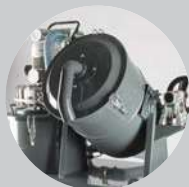
Tilting hopper for chips easy discharge
