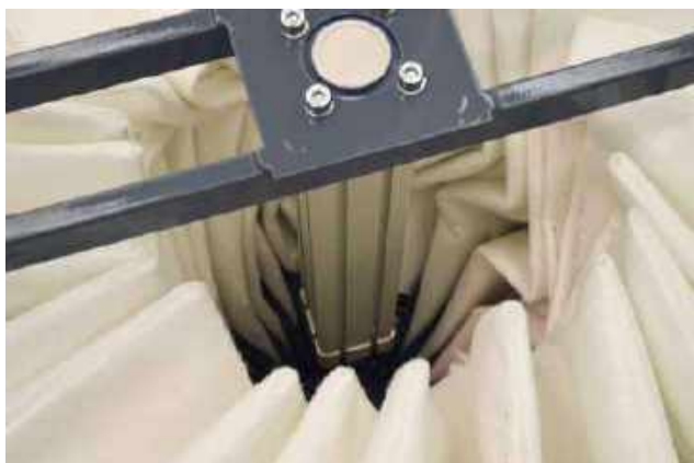
AUT: Scuotifiltro automatico. Automatic filter cleaning system
