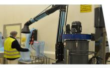
Capture particles of pigment when discharging paint powder into mixers
