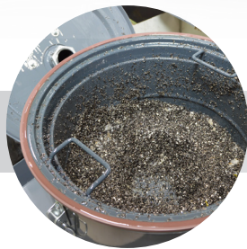
Sieve grid for the separation of swarf and metal chips from vacuumed oils
