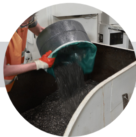
Practical discharge of swarf from the sieve grid or from the extractable collection container
